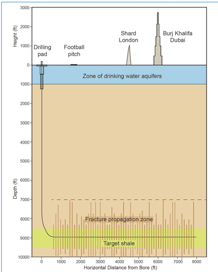
**Figure 2: True scale of a Fracking Operation**
